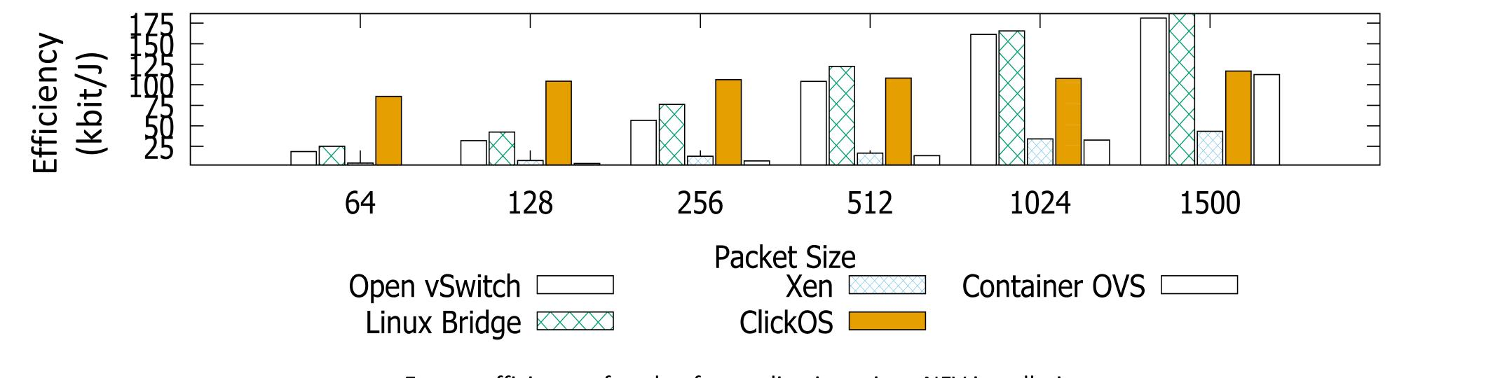
Energy efficiency of packet forwarding in various NFV installations
